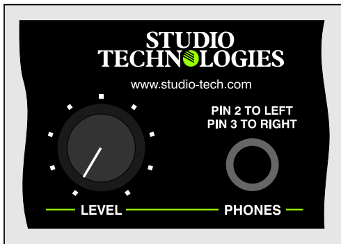
Figure 7. Detail of front panel showing headphone section
